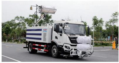
Dongfeng KR Tunnel Guardrail Cleaning Truck
